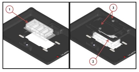
Figure 15. Magnetic lock for 1" x 2" chamber slide. To lock the slide, push simultaneously the buttons indicated with (3).
