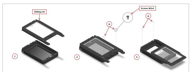
Figure 4. Assembly of the sliding lid
