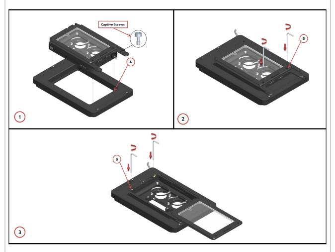
Figure 23. Connection of the Chamber with Galvo Stage
