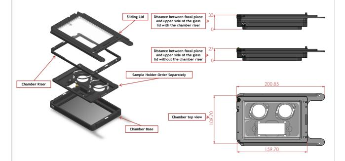
Figure 1. H301-MCL-Z100/500. Components and Dimensions.
