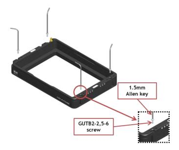
Figure 19. How to lock the Chamber Riser.
